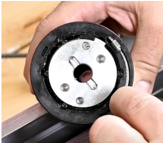
Place the Retraction Cable
