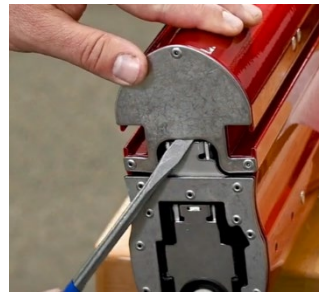
Pry off Water Shield
