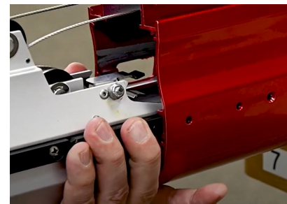
Catch Springs During Removal
