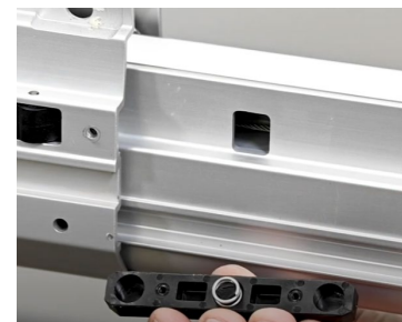
Catch Springs During Removal
