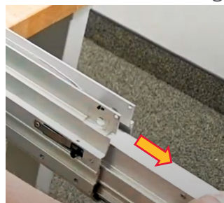
Advance the Second Stage out of the 3 rd
