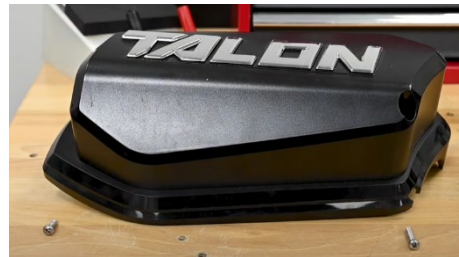
Left Motor Cover and Screws
