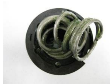
Damaged Torsion Spring
