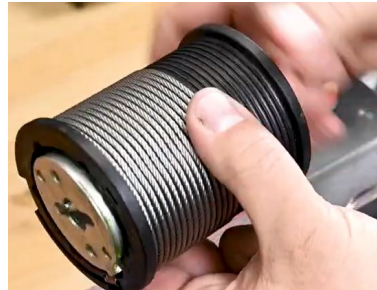
Lay the retraction cable in the grooves
