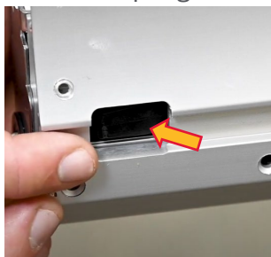
Depress the 2 nd Stage Latch
