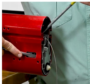
Pry Out 3 rd Stage Assembly
