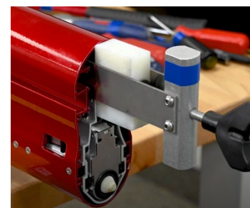
Tensioner Supported on Tool
