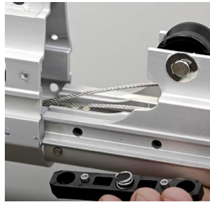
Catch the Floating GIB w/Spring
