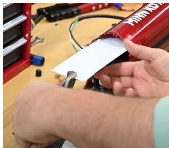
Pull The Channel Divider
