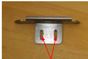
The stop sensor must be placed in these 2 nd set of holes.
