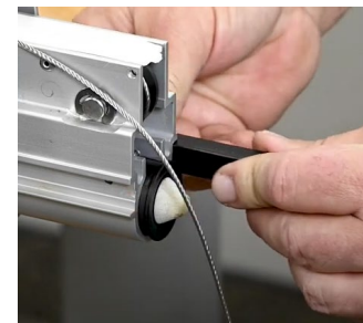
Install the Lower Fixed GIB
