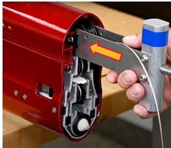
Slide the Tensioner Into Place
