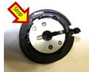
Wrap Drum/Hub Preload
