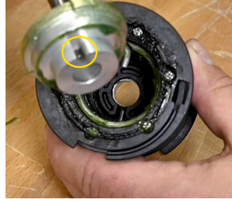
Hub Showing Hub Slot
