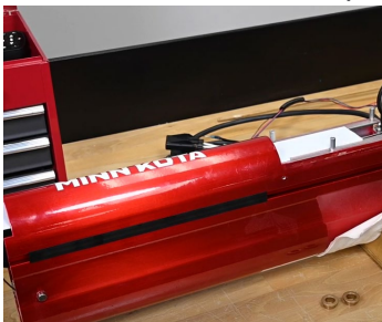
Place the Channel Divider
