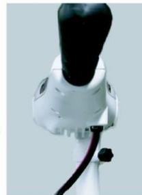
**NOTE: SUPPORT THE LOWER UNIT FOR THE FOLLOWING STEPS. LOOSENING THE DOOR CLAMP SCREW WILL ALLOW THE MOTOR TO FALL UNTIL THE HANDLE HITS THE MOTOR MOUNT IF NOT SUPPORTED.**
