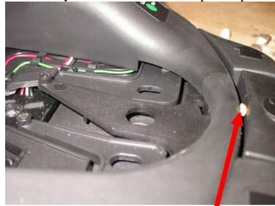
Rock stuck between button and cover.
