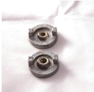
Future Orders of these two parts will be replaced by kit 2773100 or 2773101 which consists of the standard prop nut and an instruction sheet stating: ***Minn Kota no longer offers a sacrificial anode. This is due to recent environmental regulations, and the confidence in our saltwater coating and painting process, eliminating the need for the anode.***
