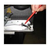
The Cam Arm is located on the right (starboard) side of the Base Extrusion behind the Motor Ramp. Remove the Right Sideplate and Motor Ramp to inspect the Cam Arm as shown in Image A.
