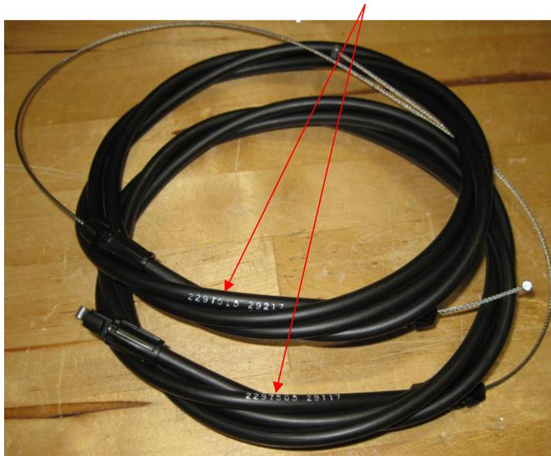
While these steering cables are approved on the Ultrax models, they have not been tested and approved for use on Fortrex, Maxxum, Maxxum Pro, Edge, and All Terrain. Continue using 2267505 and 2267515 on these models.
