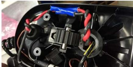
**Notice:** The red/black wires should be twisted three times on both the coil cord and brush leadwire sides and then the insulator or shrink tube is slid in place over the spade connectors. This picture shows an Ulterra, but the wire routing is similar and critical for all motors with i-Pilot systems.
