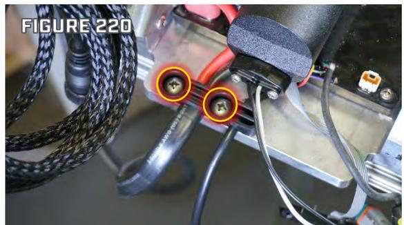
Step 17. Use a #2 Phillips Screwdriver to remove the four Screws fastening the Main Control Board to the Base Extrusion. Set these four Screws aside for use during reassembly.
