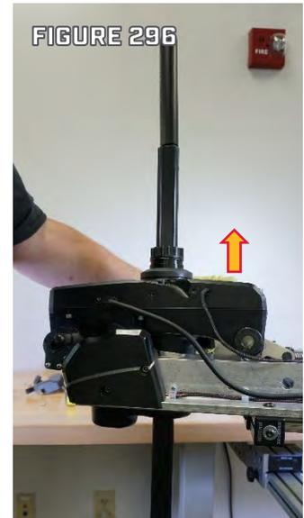
Step 5. With the Pivot Pin Removed, lift the Steering Housing off of the Lower Unit/Shaft Assembly. (Figure 296)
