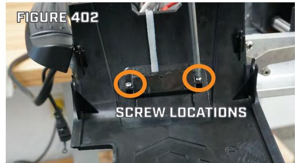
Step 14. With the Stow Deploy Lever in the vertical position use a 5/32" Allen Wrench to remove the Shoulder Bolts on the Port and Starboard side of the Stow Deploy Lever. The Shoulder Bolt on the Starboard side is the longer of the two. Push the Motor Ramps up into the stowed position, so the Latch Pin doesn't engage with the Base Extrusion later in the process of removing the Steering Housing. (Figure 403 & 404)
