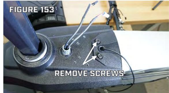
**ULTREX STEERING HOUSING INSTALLATION**
