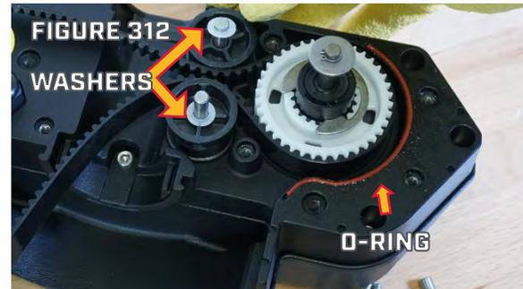
Step 8. Verify the O-Ring is in place next to the Output Gear. If the O-Ring is not sitting in its groove a small amount of
