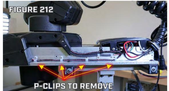
Step 9. Remove the P-Clips on the Right side of the Base Extrusion that retain the wires for the Cam/Pin Sensor. Set the P-Clips and Screws aside for use during reassembly. (Figure 213)
