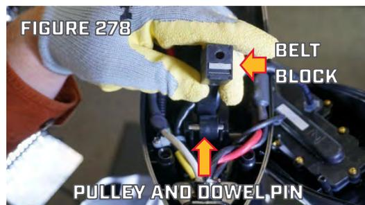
Step 7. Place the Pulley on the Dowel Pin. Place the Pulley and Dowel Pin so it rests in the groove in the Control Box (Figure 278). Feed the Belt Block Assembly down into the space between the Power and Communication Wires coming from the Coil Cord. (Figure 279)
