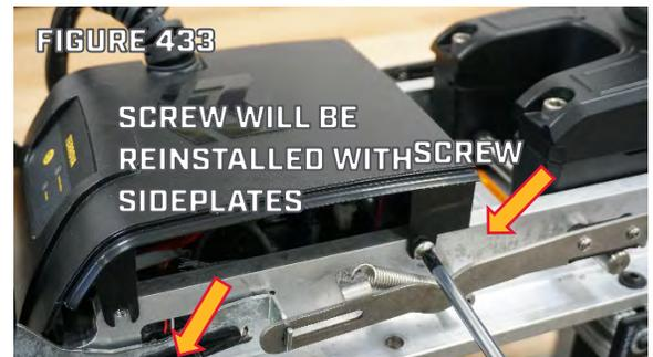
Step 10. Using a #3 Philips Screwdriver reinstall the Screws holding the Sideplates on the Port and Starboard sides of the Base Extrusion. (Figure 434)
