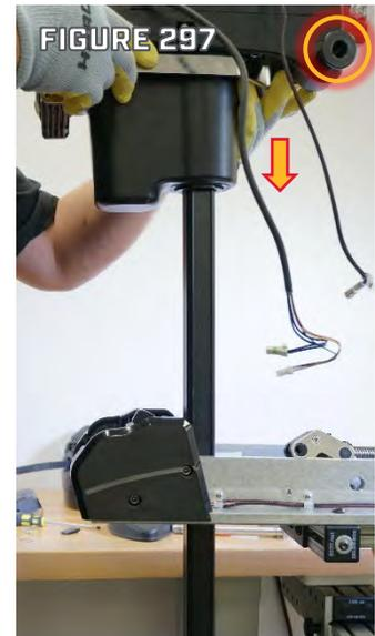
Step 3. Align the holes at the back of the Steering Housing Assembly with holes in the Base Extrusion and push the Pivot Pin through the Base Extrusion, Steering Housing, and Tilt Arms. (Figures 298 and 299)
