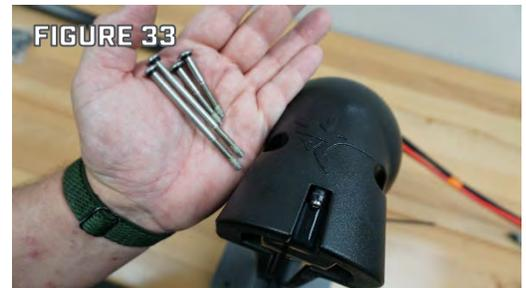
Step 4. Remove the Sonar End from the Motor Assembly.
