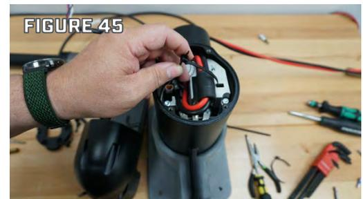
Step 6. Apply a zip tie securing the ferrite bead to the strain relief. (Figure 45)
