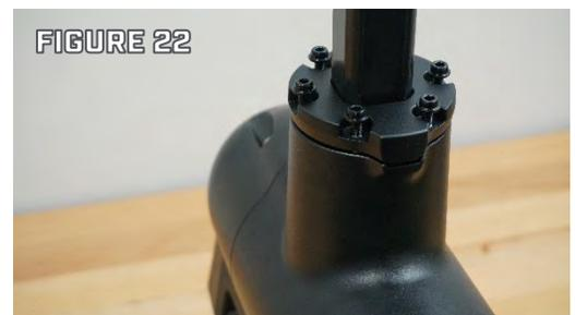
Step 10. Use a torque wrench set to 40 in-lbs or 4.5 Nm to finish tightening the clamp screws. Tighten a screw to the correct torque, then do the same for the screw directly across from it, torque a different pair, then do the last pair. (Figures 23 & 24)
