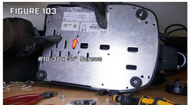
Step 19. Install the 12 #8-18 x 5/8" Screws securing the Bottom Plate to the Foot Pedal Base. These are the 12 unmarked holes in figure 103. Use hand tools and take care to follow the threads that were created on first installation of the screws to avoid damaging the foot pedal lower.
