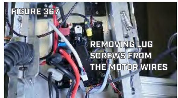
Step 14. Use #2 Phillips Screwdriver to remove the Lug Screws from the power wires. Remove wires from the wire pocket and reposition so the wires are clear of the Main Control Board.
