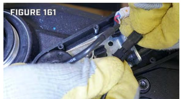
Step 10. Place the Steering Positing Sensor Cable and Steering Motor Wire Cable in the support yoke that part of the Cable Housing Bottom, then route both cables in the depression in the upper rim of the Cable Anchor Bracket between the Foot Pedal Cables. Verify the screw bosses are clear so no cables will be pinched when the Cable Housing Cover is installed. (Figure 162)
