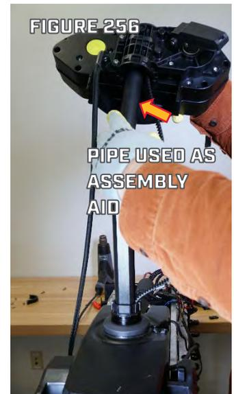
To continue with replacing the Trim Housing continue to [INSTALL TRIM HOUSING TO MOTOR](#) on Page 98.
