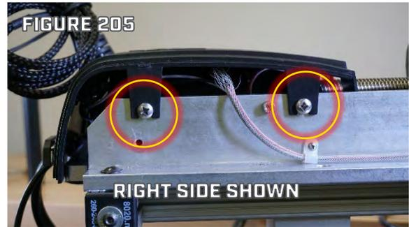
Step 2. Use a #2 Phillips Screwdriver to remove the two Screws that fasten the Power Button/LED Board to the Control Housing. Set the Screws and Control Housing aside for use in reassembly. (Figure 206)
