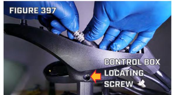
Step 6. Use a #2 Phillips Screwdriver remove the Control Box Locating Screw that secures the Control Box to the top of the Motor Shaft. (Figure 397)
