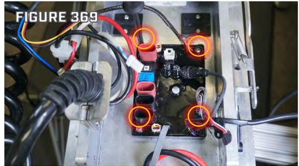
Step 2. Use the **WIRING DIAGRAM** on Page 18 to locate the correct wire pocket for the Battery + (Red) and Battery - (Black) Power Wires. Use a #2 Phillips Screwdriver Bit with a Torque Driver set to 15 in-lbs/1.7Nm to install the Lug Screws through each of the Power Wire Terminals into the Main Control Board. (Figure 369 & 370)
