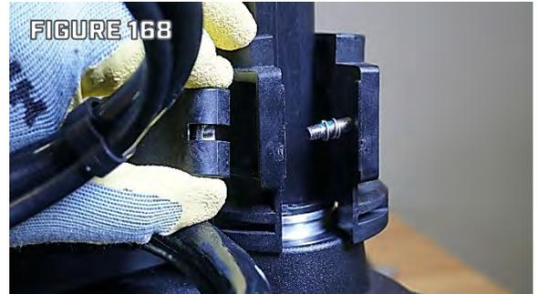
Step 17. After the Screw is three to four turns into the Cam Lock Pin close the Cam Lock Lever and use the #3 Phillips Screwdriver to fully tighten the Screw and Cam Lock Collar. Figure 169)
