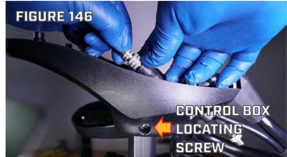
Step 6. Use a #2 Phillips Screwdriver remove the Control Box Locating Screw that secures the Control Box to the top of the Motor Shaft. (Figure 146)
