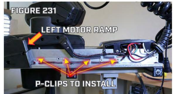
Step 12. Use a 3/16" Hex Key/Allen Wrench to Reinstall the Left Motor Ramp. (Figure 231)
