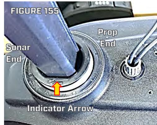
Step 2. Slide the Steering Housing onto the Motor Mount. After the Steering housing has been positioned onto the Motor Mount use ¼” Hex Key/Allen Wrench to install the two 5/16-18 x 2.25 Screws with a Lock Washer Assembly on each screw. (Figure 156)
