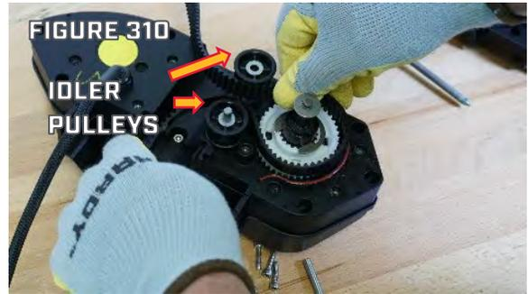
Step 6. Fold the new Belt in half with a loop towards the Drive Gear. Then, position it between the Idler Pulleys and lower the Idler Pulleys and Belt into the Trim Housing, ensuring the Belt lines up with the Drive Gear, with one belt tooth per gear tooth. (Figure 311)
