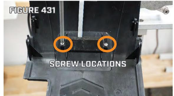
Step 8. Line up and slide the slots in the Control Housing onto the loosened Screws in the Base Extrusion. (Figure 432)
