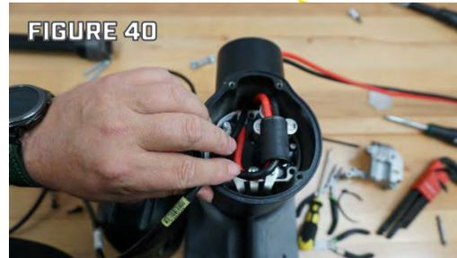
Step 2. Feed the Motor Communication Wire through the bung into the front end of the Motor Assembly. (Figures 41 & 42)
