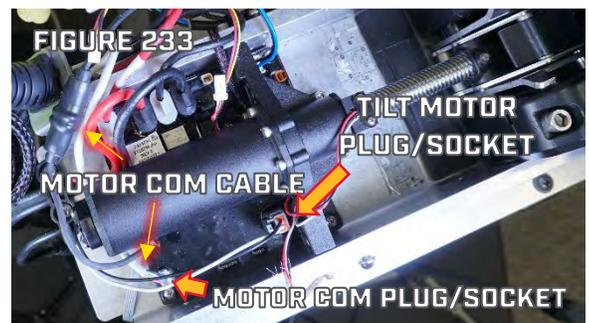
Step 15. Route the Motor Communication Cable under the Tilt Motor and plug the Motor Communication Plug into its Socket. (Figure 233)
