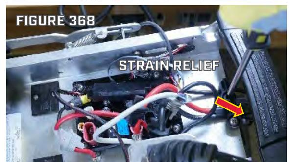
Step 16. Use #2 Phillips Screwdriver to remove the four Screws that secure the Main Control Board to the Base Extrusion and remove the Main Control Board. Set the Screws aside for use during installation.
