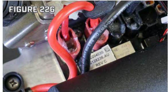
Step 7. For each of the Motor Power Leads and Battery Power Leads slide the Terminal Seals down the wire and seat them in the Terminal Pocket. (Figure 227)
