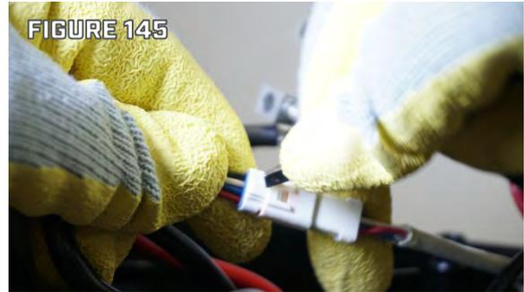
Step 5. Disconnect the Sonar Connector in the Control Box. Grip both sides of the Connector and turn them counterclockwise relative to each other to loosen the locking feature of the Sonar Connector, after connectors are loose pull the Sonar Connector apart. (Figure 146)
