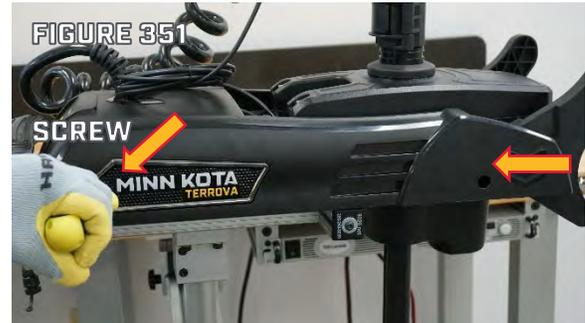
Step 2. Use a #3 Phillips Screwdriver to loosen the two Screws securing the Control Housing. It is not necessary to remove these Screws, loosening about two turns will allow the Control Housing to be removed. (Figure 352)
