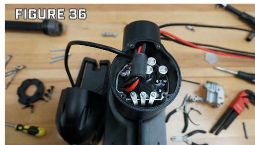
Step 9. Feed the Com Wire out of the Lower Unit Assembly to make space for the Sonar Connector to pass through the Bung. (Figure 37)
