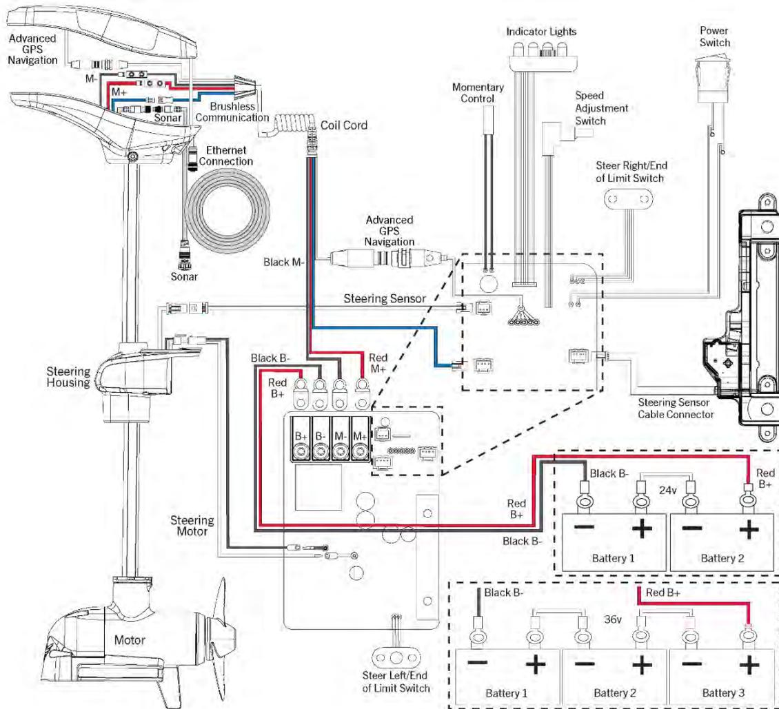
**NOTICE:** This is a multi-voltage diagram. Double-check your motor's voltage for proper connections. Over-Current Protection Devices are not shown in this illustration.
