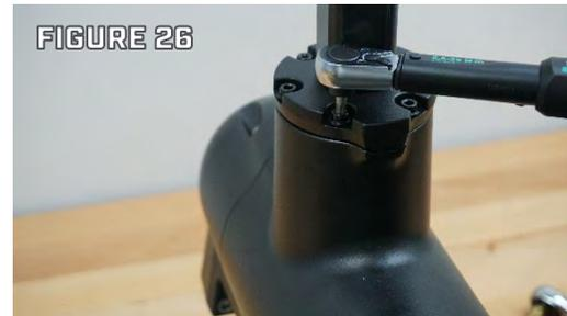
Step 12. Return the Lower Unit/Shaft to the Motor Assembly.
