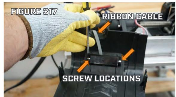
Step 4. Use a #3 Philips Screwdriver to remove the two Screws securing the Strain Relief to the Base Extrusion. (Figure 318)
