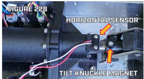
**NOTICE:** Route the sensor wires as shown in Figure 228. Over the Tilt Actuator. This routing avoids any pinch points the wires otherwise may contact.
