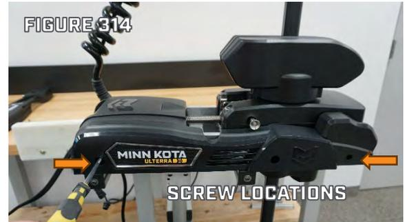
Step 2. Using a #3 Philips Screwdriver, loosen the four Screws that secure the Control Housing to the Base Extrusion by 1-2 turns. The Screws only need to be loosened and not completely removed. Carefully lift the Control Housing from the Base Extrusion to prevent damaging the Ribbon Cable for the Power Button. The four Screws can remain installed in the Base Extrusion. (Figure 315 & 316)
