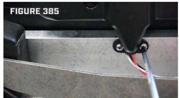
Step 16. Position the Power Button Assembly in the Control Housing, use a #2 Phillips Driver to install the two Screws that were set aside during disassembly for retaining the Power Button Assembly in the Control Housing. (Figure 386)
