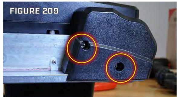
Step 6. Use a #1 Phillips Screwdriver to Remove the two Screws that fasten the Cam/Pin Sensor to the Base Extrusion. Set the Screws aside for use during reassembly. (Figure 210)
