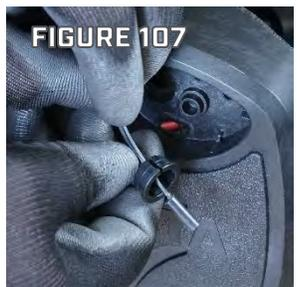
Step 25. Place the momentary button spring onto the protrusion that supports the spring in the Momentary Button Cavity. Place the shorter tab of the Momentary Button into the corresponding slot adjacent to the Momentary Button Cavity, guide the longer tab onto the opposite wall of the Momentary Button Cavity then push the Momentary Button down until the longer tab catches. (Figure 108)
