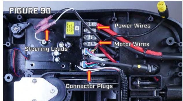
Step 21. The three connector plugs are closely grouped in the corner of the control board. Use a small flat-blade screwdriver or pick to depress the locking tab on each while pulling the plug body free of the control board. Be aware that the motor communications wire and the steering sensor wire use the same type of plug. The motor will not function if these are reversed during assembly. Refer to the included Wiring Diagram for connector locations.
