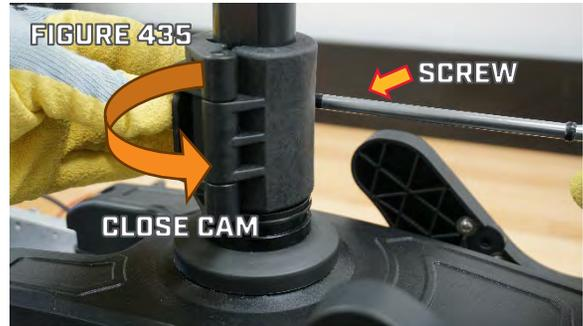
Step 12. Models that have a 72", 87", or 100" Shaft will need to have the Stow Lock Collar reinstalled. The Locking Tab will need to be in the straight forward position. Use a #2 Phillips Screwdriver to tighten the four Screws. The back half of the Stow Lock Collar has four Nuts you will want to make sure didn't fall out. (Figure 436)
