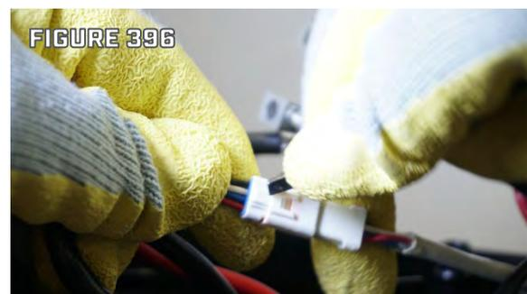
Step 5. Disconnect the Sonar Connector in the Control Box. Grip both sides of the Connector and turn them counterclockwise relative to each other to loosen the locking feature of the Sonar Connector, after connectors are loose pull the Sonar Connector apart. (Figure 397)
