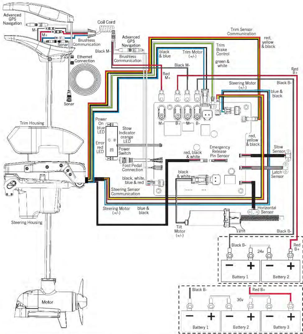
**NOTICE:** This is a multi-voltage diagram. Double-check your motor's voltage for proper connections. Over-Current Protection Devices are not shown in this illustration.
