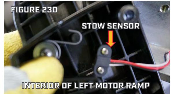
**NOTICE:** The raised detail and writing on the face of a Hall Effect Sensor indicate the direction of the Hall Effect Sensor. The Sensor is activated by the South Pole of Magnet arriving in close enough proximity to the Hall Effect Sensor. The directions above point the Sensor in the direction the magnet that actuates the Sensor will approach from. Double check that at each of the three Sensors the Sensors are facing the associated Magnets.
