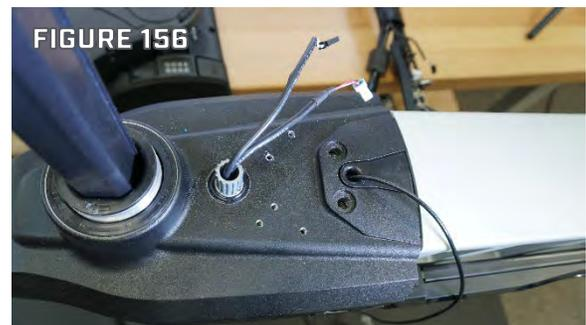
**NOTICE:** The Foot Pedal Assembly may be installed from the left or right of the Steering Housing based on user preference. Use the same orientation that was in use on the replaced steering housing. As shown is from the right; this is the factory standard orientation.
