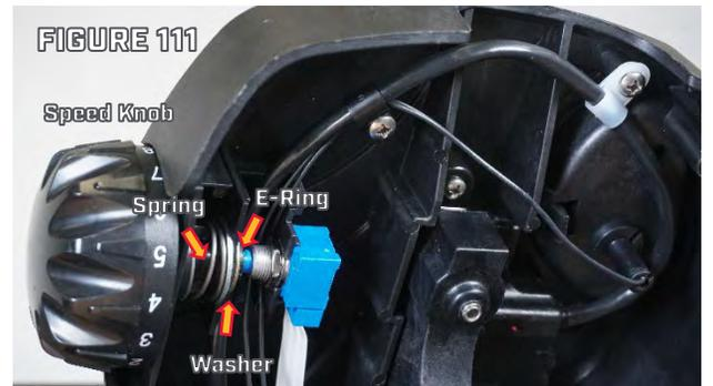
Step 30. Push the E-ring onto the groove of the Speed Selector Knob to secure the Speed Selector Knob in place. (Figure 111)
