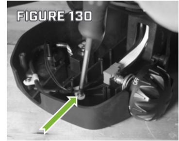
Step 3. Route the steering sensor board cable through the small opening where the potentiometer ribbon cable and reed switch wires are located.
