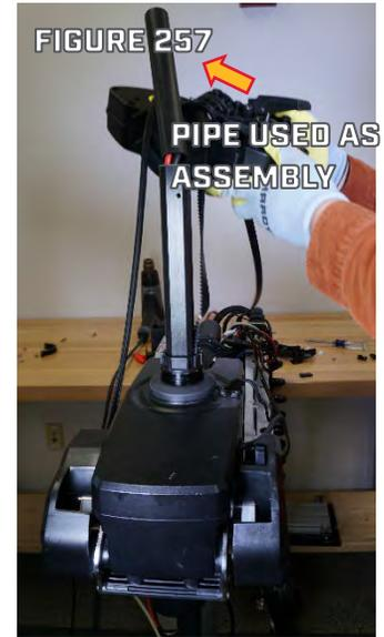
Step 2. Lift the Motor Lower Unit and Motor Shaft 15". Tape the end of the Belt to the Motor Shaft in the Belt Groove just above the Steering Housing. Return the Motor Lower Unit/Motor Shaft to the floor, the Belt will be pulled through the steering housing by the Masking Tape. (Figure 258). Remove the Masking Tape.
