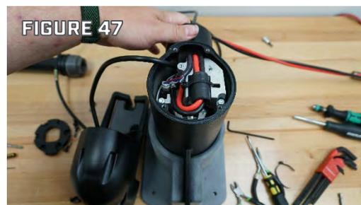
Step 8. Position the Red Motor Lead in its groove in the strain relief.
