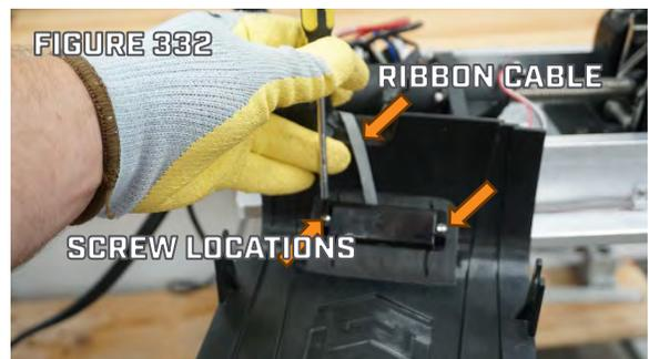
Step 19. Line up and slide the slots in the Control Housing onto the Screws in the Base Extrusion if not removed in Step 2. Use a #3 Philips Screwdriver to tighten the four Screws that were previously loosened 1-2 turns in Step 2. (Figures 333 & 334)
