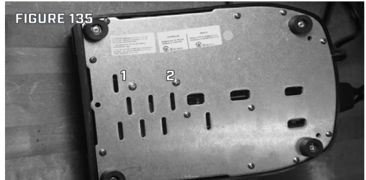
**NOTICE:** Ensure that the wires in the foot pedal are properly routed and will not be pinched or damaged while installing the bottom plate.
