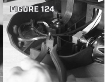
Step 4. Disconnect the control board potentiometer from the speed control knob, loosen the potentiometer nut completely using a 1/2" open-end wrench, and slide it out. (See Figures 125 & 126)
