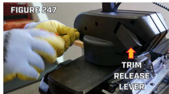
Step 2. Pull the belt downward creating at least 4" of Belt slack between the Steering Housing and Lower Unit, this slack is necessary for step 16. If the belt will not travel freely through the Trim Housing pull the Trim Release Lever back open. (Figure 248)
