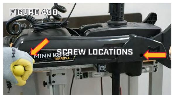
Step 12. Using a #3 Philip Screwdriver loosen the Screws one or two turns, that secure the Control Housing to the Base Extrusion. There is only one Screw on each side as the other two Screws are removed when the Sideplates are taken off. (Figure 401)
