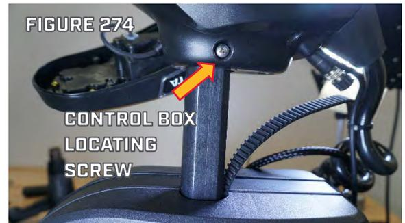
Step 2. Place the Nut that was removed from the Control Box during disassembly in the hex shaped detail on the right side of the Control Box. Insert the Control Box Locating Screw through the Control Box and the hole in the Motor Shaft and tighten the control Box Locating Screw into the Nut. (Figure 274).
