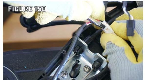
Step 14. On the toe end of the Foot Pedal Assembly, use a #3 Phillips Screwdriver to loosen the Cable Tension Screw several turns. The tension must be loosened to allow removal of the wrap drum from the steering output. Be careful to not fully remove the Cable Tension Screw. (Figure 151)
