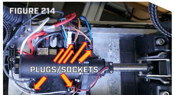
**NOTICE:** If the Trim Position Sensor Plug does not have a visible red mark use a Red Permanent Marker to add a visible Red Mark to the Plug. The Trim Position Sensor Plug and Steering Position Sensor Plug are identical other than that mark, mixing them up during reassembly may result in damage to the motor during calibration.
