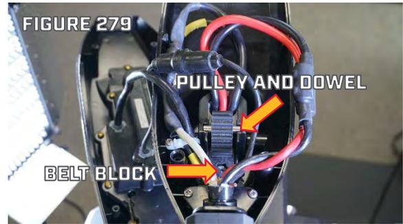
Step 8. Insert the Belt Tensioning Screw with Washer through the hole in the bottom of the Control Box. Engage the Belt Tensioning Screw into the Nut in the Belt Block. It may help to hold the Belt Block down with a free hand to get the Tensioning Screw Started into the Nut. Use a 5/32" Hex Key to tighten the Belt Tensioning Screw to a torque of 10 in-lbs/1.1nM. (Figure 280).
