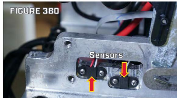
Step 11. Use a T10 driver to install the #4-40 Screws, two to each Sensor, that secure the Sensors to the Base Extrusion.
