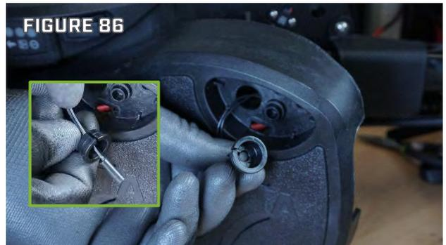
Step 13. Pull the reed switch through the hole the reed switch clip was secured. The reed switch and the potentiometer should be loose under the foot pedal rocker.
