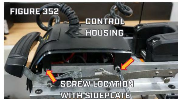
Step 3. Use #2 Phillips Screwdriver to remove the two Screws securing the Power Button Assembly to the Control Housing. Set these Screws and the Control Housing aside for use during reassembly. (Figure 353)
