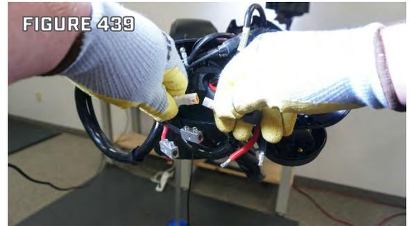
Step 16. Center the Heat Shrink on the connector, the ends of the Heat Shrink should be on the outer jacket of the cable, no small conductors should be visible.
