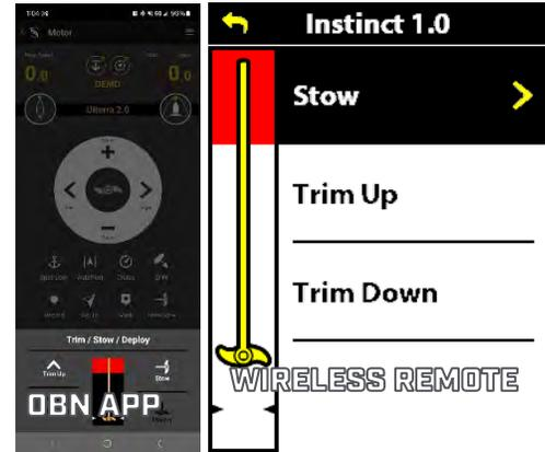
**NOTICE:** If the Tilt Disconnect Pin has been pulled you may need to push down on the Tilt Bracket to engage the Latch Pin to the point the Latch Sensor is engaged. When the sensor is properly located the Ulterra or Instinct menu in the OBN App or Wireless Remote, will have options “Trim Up, Trim Down, and Stow”, “Deploy” will not be present on the remote and will not be selectable in the OBN App (FIGURE 201)
