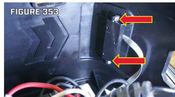
Step 4. Remove the Stow/Deploy Lever to access the two Sensors. The following steps explain removal of the handle assembly.
