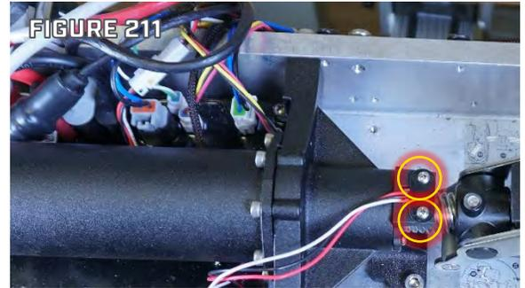
Step 8. Remove the four P-Clips on the left side of the Base Extrusion that retain the wires for the Plunger Sensor. Set the P-Clips and Screws aside for use during reassembly. It is not necessary to remove any of the P-Clips from the Steering and Trim Cables. (Figure 212)
