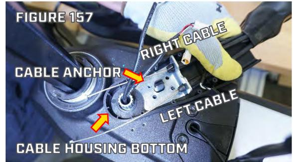
Step 4. Use #2 Phillips Screwdriver to install the three #10-24 Screws Securing the Cable Anchor Bracket and Cable Housing Bottom to the Steering Housing. (Figure 157)
