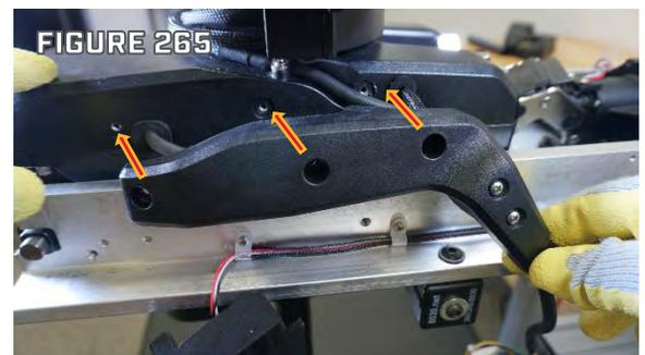
Step 8. Route the Trim Housing and Steering Housing Cable Assemblies in the Four P-Clips then use a #2 Phillips Screwdriver to fasten the P-Clips to the Base Extrusion. (Figure 266).
