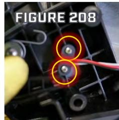
Step 5. Use a 3/16" Allen Key to remove the two Screws that fasten the Right Motor Ramp to the Base Extrusion. Set the Motor Ramp and Screws aside for use during reassembly. (Figure 209)
