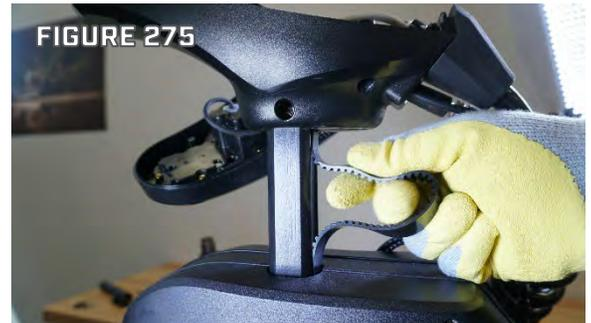
Step 4. Insert the Belt into the Upper Belt Block from the end with the captured Nut and with the teeth of the Belt facing up. Feed the Belt completely through the Belt Block. (Figure 276)
