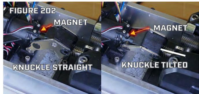
**NOTICE:** If the Tilt Disconnect Pin is not installed the Horizontal Sensor may be tripped. This will result in error 3.6, the red light on the motor will flash. The error code can be viewed via the OBN app or Wireless Remote. To proceed rotate the Tilt Knuckle so the magnet is slightly away from the Stow Sensor. (Figure 202)
