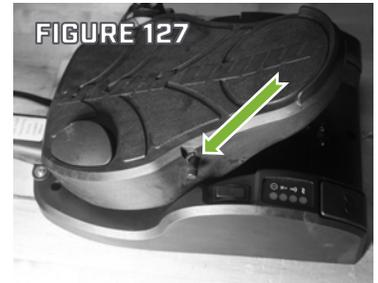
Step 6. Place the foot pedal upper rocker on a flat surface so the underside is visible. The Lower Rocker, still connected to the steering cables, stays in the foot pedal base (As shown in Figure 128).
