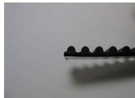
Belt cut properly in valley
