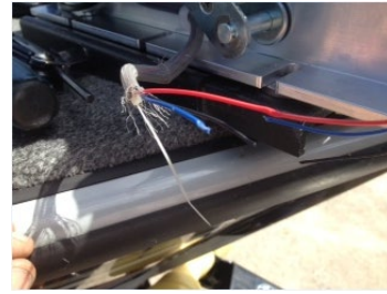
Actual photo supplied by a service provider showing damage caused by improper rigging.
