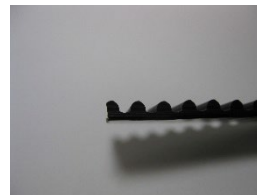
improperly cut lift belt
