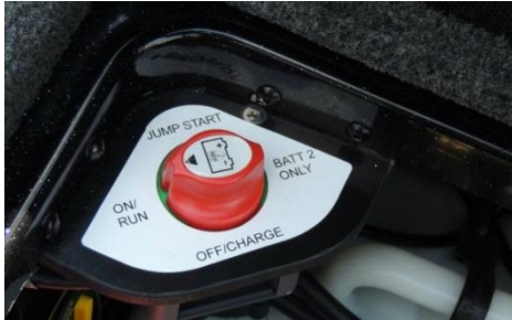
Figure 1: Battery Selector Switch
