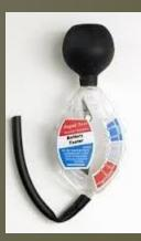
With the battery at a temperature of 77-80° F the specific gravity of the electrolyte in a fully charged battery will be 1.265 or slightly higher. Specific gravity readings should not vary more than .05 between cells.
