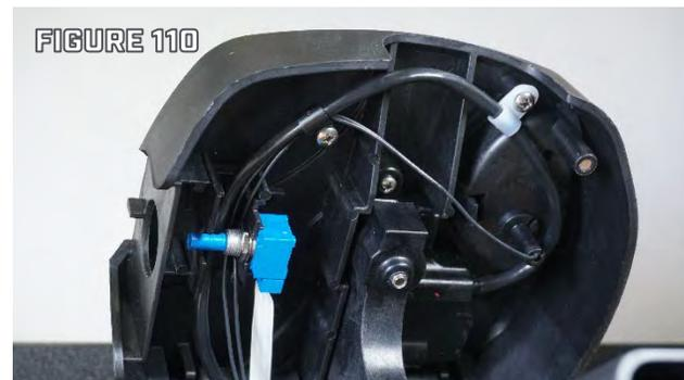
Step 28. Use the 1/2" wrench to tighten the Potentiometer Nut. (Figure 110)
