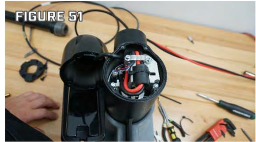
Step 3. Use a #2 Phillips to remove the two screws securing the Top Cast to the Strain Relief
