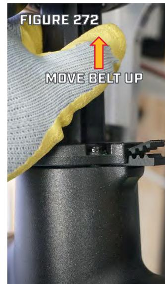
Step 4. Remove the Belt slack below the Steering Housing by Pulling the Belt through the Trim Housing until the Lower Unit starts to raise up. If the Belt does not move freely, pull the Release Lever to disengage the Trim Motor. (Figure 273)
