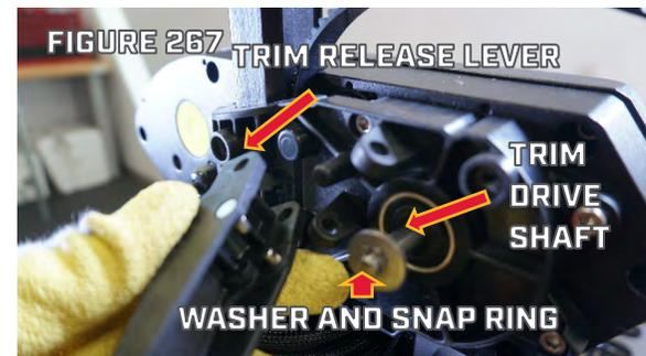
Step 10. If the Trim Release Lever fell off of the Trim Housing, slide the Trim Release Lever over the washer so the pins in Trim Release Lever are behind the Washer. Install the Trim Release Lever Dowel pin. (A small amount of Marine Grease on the Pin may be applied to keep it from falling out while installing the cover.) (Figures 267 and 268)
