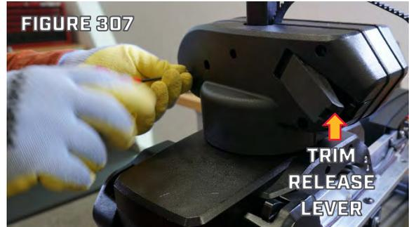
Step 6. After the new Belt has passed through the Trim housing, remove the duct tape from both sides of the Belts. Discard the old Belt.
