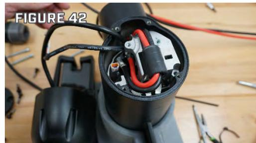
**NOTICE:** Use the Gummy Seal to properly align the wires. Any tangles, overlaps or twists will prevent the motor from being assembled correctly.
