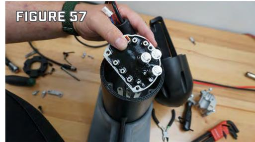
Step 12. Remove any foreign material from the mounting surface of the Inverter Board. Figure 58 shows a cleaned mounting surface.
