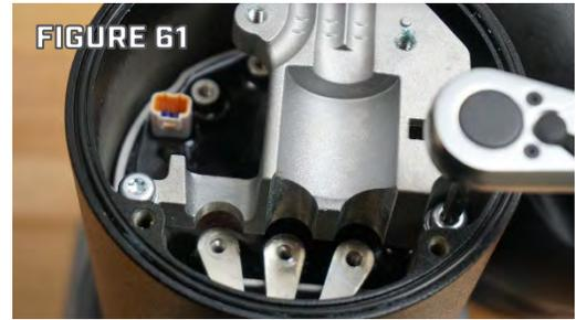
Step 17. Install the Terminals to the Phase Leads, Use an appropriate Driver Bit and a torque driver set to 15 in-lbs (1.7 Nm) to install the terminal Screws. (Figure 62)
