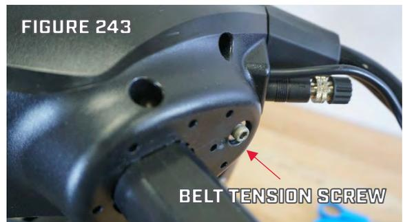
Step 6. With the Belt Tension Screw removed pull the Belt Block Pulley Wheel and Dowel Pin out the Control Box. The Motor Power Wires, Communication Cable and Transducer Cable will likely need to be moved out of the way to complete this process. (Figure 244).
