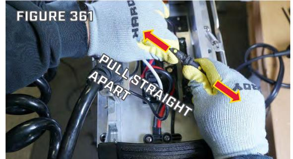
Step 9. Depress the locking tab on the Plug for the Steering Motor, then pull the Steering Motor Plug from the Control Board. (Figure 362). This Plug's locking tab can be released by hand, without tools.
