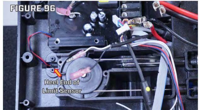
**NOTICE:** Be sure to push the End of Limit Sensors through the foot pedal base so they will not fall back through when you turn the Foot Pedal Assembly over.
