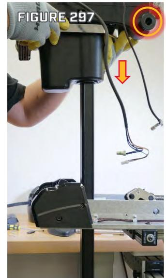
Step 3. Align the holes at the back of the Steering Housing Assembly with holes in the Base Extrusion and push the Pivot Pin through the Base Extrusion, Steering Housing, and Tilt Arms. (Figures 298 and 299)
