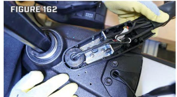
Step 11. Place the Cable Housing Top over the Cables, Wrap Drum, Steering Motor Wires Connection, and Steering Sensor Connection. Use #2 Phillips Screwdriver to install the eight #6-19 x 1" Screws that secure the Cable Housing Top. (Figure 163)
