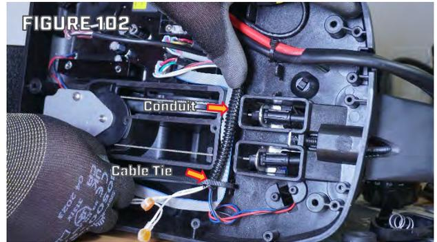
Step 16. Install the included Cable Ties so that it secures the wires for the Power Switch and Right End of Limit Sensor and the Ribbon Lead for the Indicator Light Assembly. (Figure 102)
