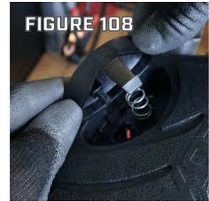
*The Calibration section will have a description of positioning the reed switch for proper function, for now the switch should be at the bottom of the Reed Switch Clip. MOMENTARY SWITCH CALIBRATION, Page 84*
