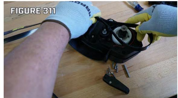
Step 7. If the Idler Pulleys were lifted far enough to displace the white plastic Washers reinstall the Washers on the Pulley Shafts. One Washer on each side of each Idler Pulley, the Washers under the Idler Pulleys should not have moved during this operation. (Figure 312)
