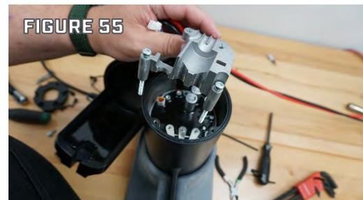
Step 11. Remove inverter. Tip the inverter up away from the phase leads for removal. (Figures 56 & 57)
