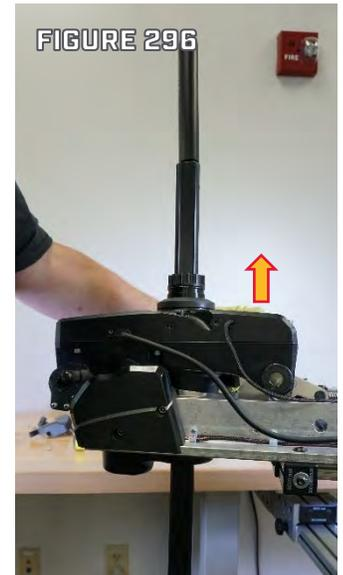
Step 5. With the Pivot Pin Removed, lift the Steering Housing off of the Lower Unit/Shaft Assembly. (Figure 296)
