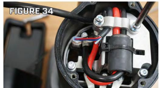
**NOTICE:** One of the screws securing the Strain Relief body is under the Com Wire.
