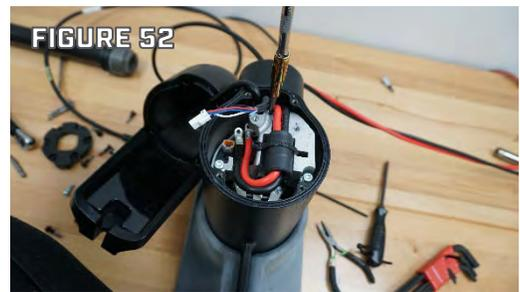
**NOTICE:** The screws securing the phase leads and power leads may either be T20 (830-120) or #2 Phillips (830-123). The #2 Phillips screws may also be driven with a 7mm Socket, but due to close clearance standard 7mm sockets may not be used at all screw locations.
