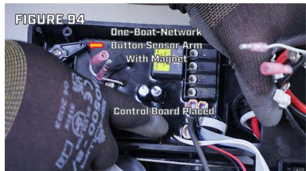
Step 3. Routing the End of Limit Sensors. The two End of Limit Sensors are the Hall Effect Sensors attached to the Control Board. One of the two Hall Effect Sensors will have a mark on the back side of the sensor. The marked sensor is the Left End of Limit Sensor and is installed at the heel end of the pedal. The toe/Right End of Limit Sensor is also closer to the toe side of the control board than the heel/left sensor (Figure 95).
