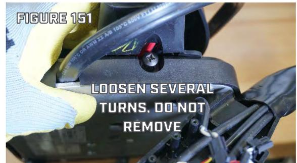
Step 15. Make note of which side of the Steering Housing the Foot Pedal Assembly is installed on (Left/Right). With the motor pointed straight ahead use a marker on the Wrap Drum and Cables Housing Bottom to record current alignment. Cable orientation may be changed by the user, the marks will be used during reassembly to maintain the user setting.
