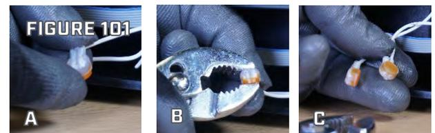
Connector, then use a slip jaw pliers to close the connector onto the wires. When fully closed grease will push out of the holes around the wires and the button will be flush with the body of the switch.
