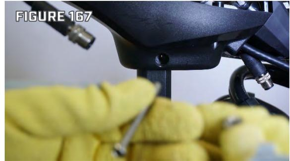
Step 16. Position the Depth Collar onto the Steering Housing. Slide the Screw through the Depth Collar Bolt Half and Spring. Close the Depth Collar Cam Half over the Spring and Screw. Verify the Cam Lock Pin is within the Cam Lock Lever, align the threads of the Cam Lock Pin with the Screw, use #3 Phillips Screwdriver to start the Screw into the Cam Lock Pin. Do not Fully tighten the collar. (Figure 168)
