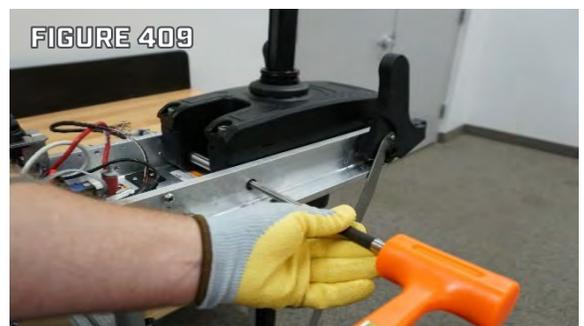
Step 19. After removing the Pivot Pin, slide the Steering Housing up and off of the Shaft. The Steering Housing has two Bushings, one on each side of the Steering Housing, where the Pivot Pin was removed. Set the Bushings aside for reuse during installation. (Figure 410 & 411)
