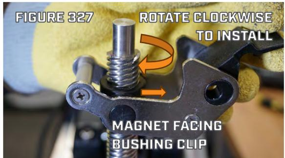
**NOTICE:** Figure 327 and 336 show the magnet facing up toward the Bushing Clip which is the correct orientation on the Tilt Bracket Assembly. If the magnet isn't facing up the Motor will not trim back onto the Motor Ramps during the stow sequence. The Motor will stay trimmed out 6" until the magnet is correctly oriented.
