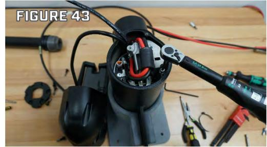
Step 4. Apply Loctite to the threads of the three screws securing the Strain Relief to the Motor Housing. (Figure 44)
