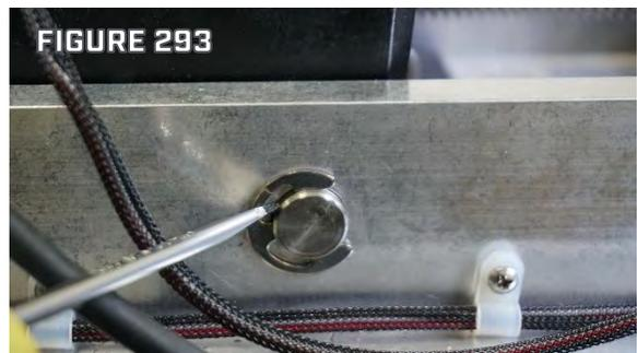
Step 4. Drive the Pivot Pin out of the Base Extrusion with a punch or screwdriver. (Figures 294 & 295)
