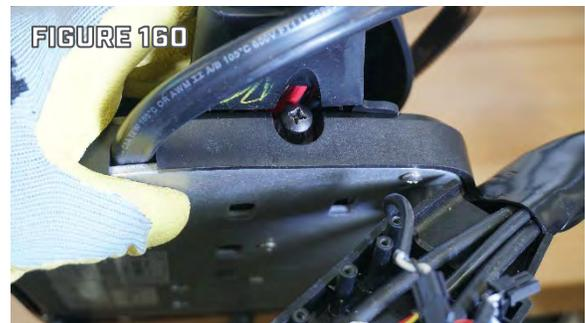
Step 8. Connect the Steering Position Sensor Cable (White Plug).
