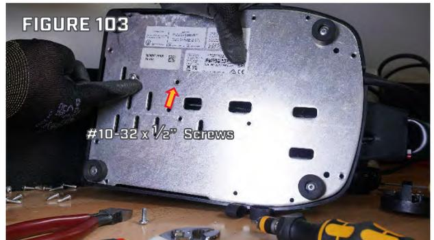
Step 18. Using the two new #10-32 x 1/2" Screws included in this kit Secure the Control Board to the Bottom Plate. In Figure 103, 10-32 x 1/2" Screw locations are indicated by arrows. One location has a screw getting inserted.
