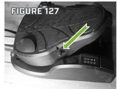
Step 7. Place the foot pedal upper rocker on a flat surface so the underside is visible. The Lower Rocker, still connected to the steering cables, stays in the foot pedal base (As shown in Figure 128).
