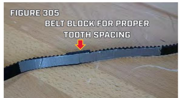
Step 4. Flip the joined Belts over, remove the Belt Block, and apply the other strip of tape to the toothed side of the two Belts, beginning at the seam between the belts and working towards the ends of the strip of tape press the tape into the teeth. (Figure 306).
