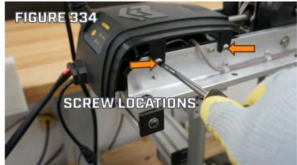
Step 20. Use a #3 Philips Screwdriver to reinstall the Port and Starboard Sideplates. (Figure 335)
