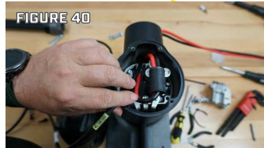
Step 2. Feed the Motor Communication Wire through the bung into the front end of the Motor Assembly. (Figures 41 & 42)
