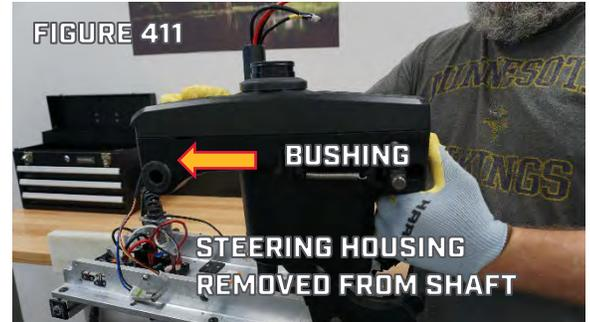
Step 20. Figure 412 shows the Steering Housing successfully removed from the Shaft.
