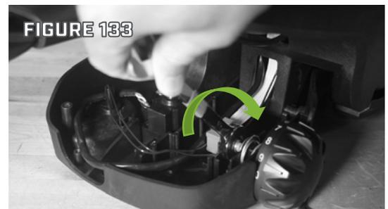
Step 6. Turn the foot pedal back over and connect the steering sensor board connector to the main control board, ensuring it clicks into place. (See Figure 134). Refer to the wiring diagrams to ensure proper installation location of the sensor plug.
