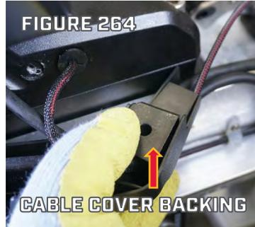
Step 7. Attach the Cable Cover to the Steering Housing using the three Machine Screws that were removed during Disassembly step 17. (Figure 265)
