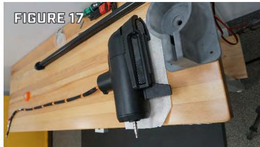
Step 4. Feed the wires into the shaft and slide the shaft assembly down the wires until the shaft plug is in contact with the motor bung. (Figures 18 & 19)
