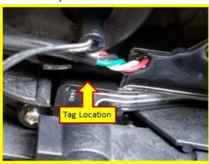
Ultrex motors with serial number R213MK#### and later are manufactured with the corrected component on the Steering Sensor Board.
